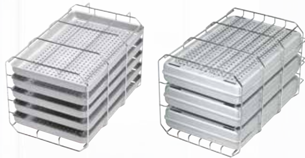
Variable loading options. By turning the tray holder 90°, 3 normal cassettes with lids or 5 trays without lids can be loaded.
